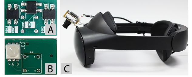
Figure 12: Hardware. (A) Front side and (B) back side of our circuit board. (C) Camera mounted on an AR headset.
