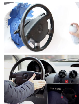
Figure 3. Electrick enables multi-touch sensing on complex objects. For instance, a touch-sensitive steering wheel can monitor drivers for safety behaviors.
