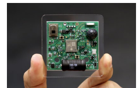
Figure 6. My general-purpose sensor board can turn into a wide variety of software-defined "synthetic sensors" such as door sensor and cooking detector.
