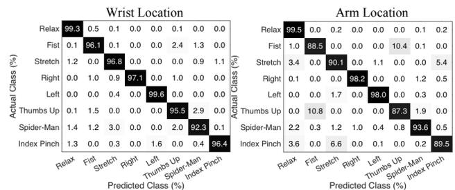
Figure 6. Confusion matrix of the hand gesture set when Tomo is worn on the wrist (left) and on the arm (right).
