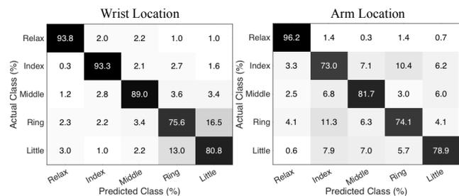
Figure 7. Confusion matrix of the pinch gesture set when Tomo is worn on the wrist (left) and on the arm (right).
