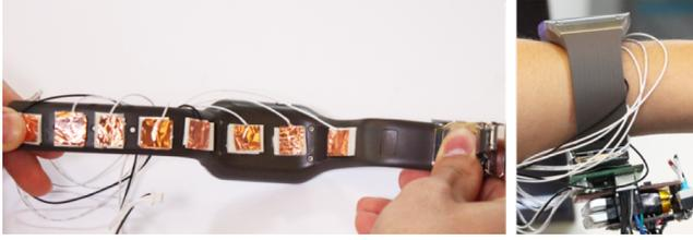
**Figure 11.** As a proof of concept, we modified a Samsung smartwatch, adding EIT sensing and real-time hand gesture recognition capabilities.
