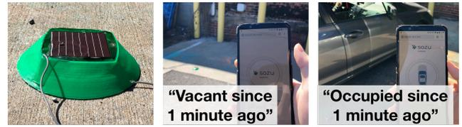
Figure 19. Sozu tag used for parking occupancy detection.
