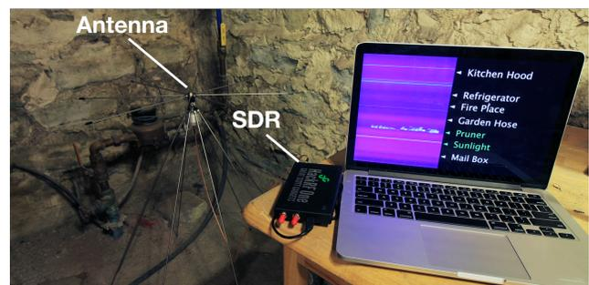
Figure 11. Sozu receiver setup deployed in a basement.
