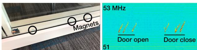
Figure 13. Strategic placement of magnets on a door frame allows the direction of a sliding door to be sensed.
