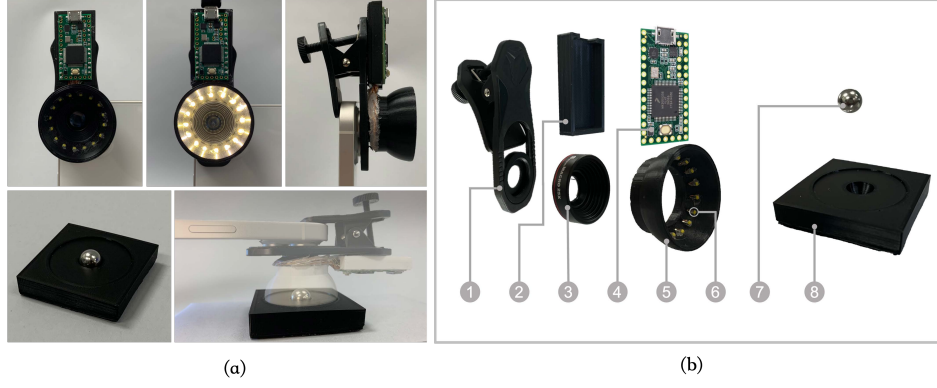
Figure 1: (a) SkinProfiler (top-left) LED light dome front view, (Middle) LED light dome all LEDs on, (top-right) LED light dome side view, (bottom-left) the calibration tool, (bottom-right) usage of the calibration tool; (b) fabrication and accessory assembly 1.camera clamp, 2.teensy holder, 3.macro Lens (25x), 4.Teensy 3.2, 5.light dome, 6.white LED, 7.stainless steel ball, 8.ball holder.
