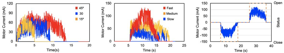
Fig. 11. Example of using *MiniKers*'s sensing capability. Left: The integral of motor current correlates door angle. Center: The speed of opening/closing the door can be inferred from the magnitude of current. Right: The direction of the current indicates the door status.
